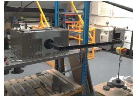
Figure 10 – Torque Testing Atlas Socket
