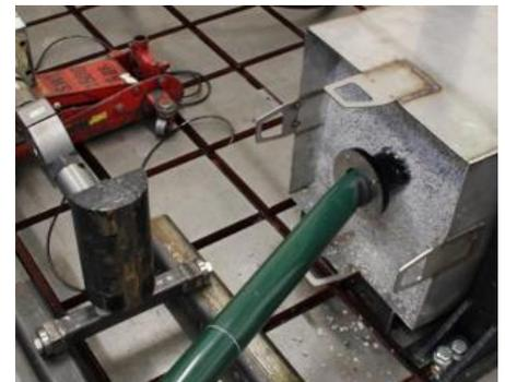
Figure 9 – Impact Loading Atlas Socket
