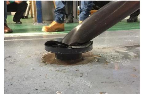
Figure 8 – Crash Testing the Atlas Socket
