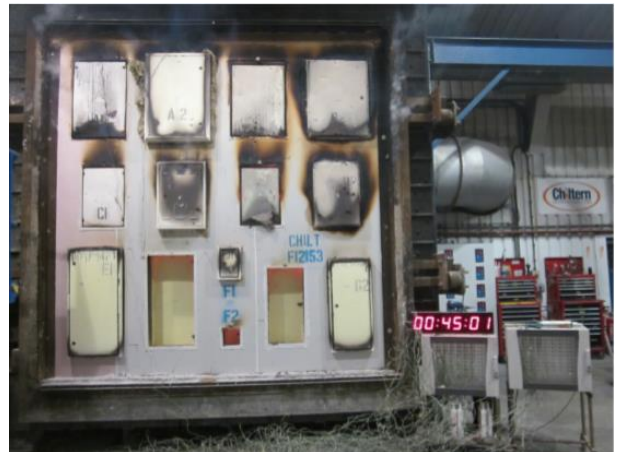
Figure 5 - Fire testing of various FireSeal products front and rear facing
