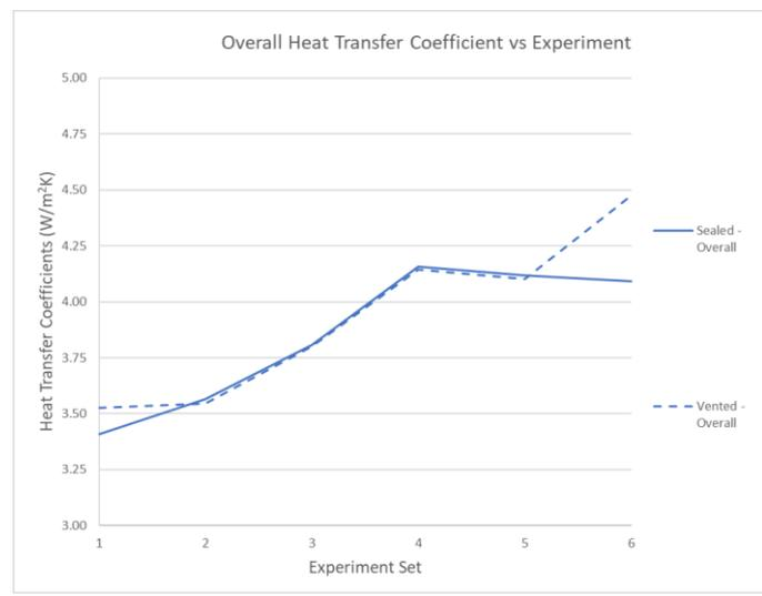
Figure 4 - Overall Heat Transfer Coefficient for each pair of experiments
