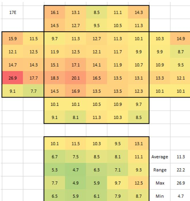
Figure 9 – Sample Heat map of sealed circulated cabinet Experiment 5a
