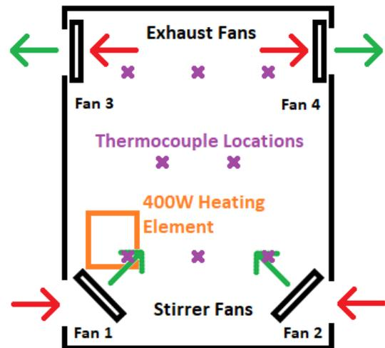
Figure 2 – Experiment diagram showing approximate fan positions, air-flow direction (red is intake, green is exhaust), thermocouple location and heating element location.
