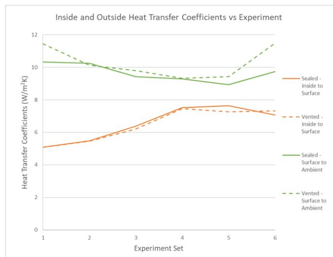
Figure 5 - Inside and Outside Heat Transfer Coefficients for each pair of experiments (Convection and Radiation components combined)
