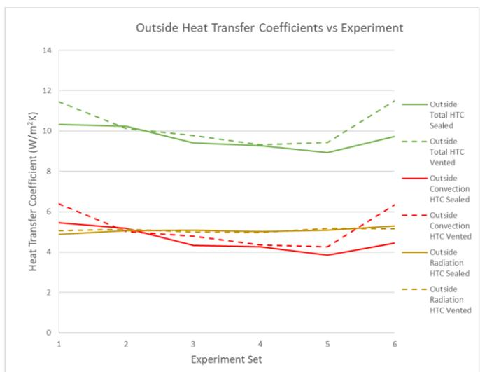
Figure 6 - Outside Convection and Radiation Heat Transfer Coefficients for each pair of experiments
